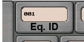
The Equipment ID may be changed by touching the [Eq. ID](#) button. Once the button is highlighted, there are two ways to change the data:
