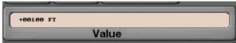
The actual value to be transmitted can be edited by selecting the **Value** button. The value is entered in decimal format. For instance to enter a value of 123.4 nautical miles for **Distance To Go**, select the **Value** button, touch **CLR** and then touch **1, 2, 3, ., 4** and then **ENTER**.
