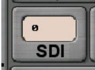
The source destination identifier can be edited by selecting the [SDI](#) button. The SDI is a two-bit portion of the word. Therefore the SDI can hold the values [0](#), [1](#), [2](#), and [3](#). The meaning of the SDI is label dependent.
