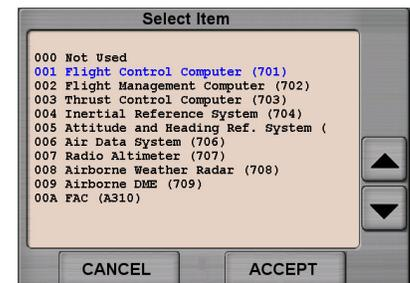
In ARINC 429, the Equipment ID is a three digit hexadecimal number. Therefore, the hexadecimal keys are enabled on the keypad.
