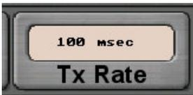
The interval at which the current label will be transmitted may be set using the [Tx Rate](#) button. The interval can be selected to be from **1** to **99,999** msec.
