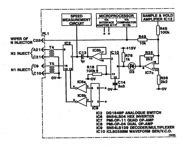
Speed Injector Circuit Figure 10
