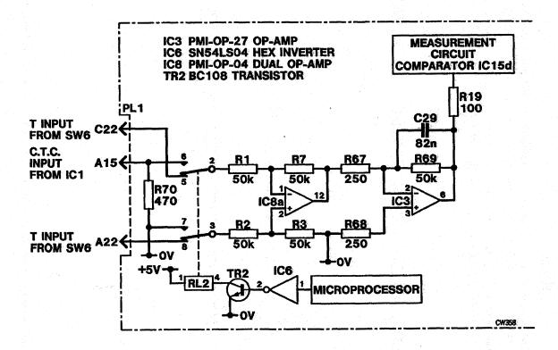
Thermocouple Input Measurement Circuit Figure 11
