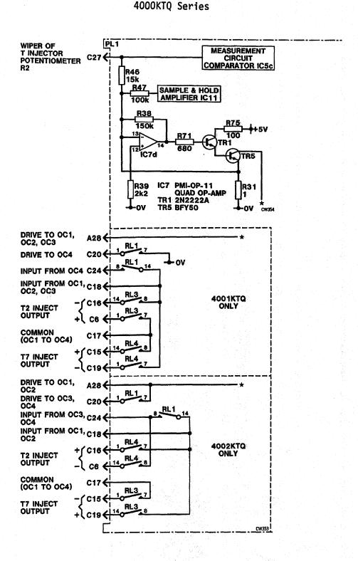
Thermocouple Injector Circuit Figure 12
