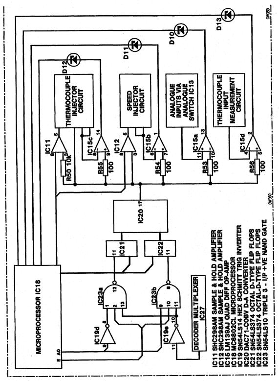
Microprocessor Analogue Interface Circuit Figure 17
