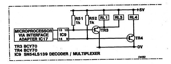
Thermocouple Injector Relay Drive Circuit Figure 13
