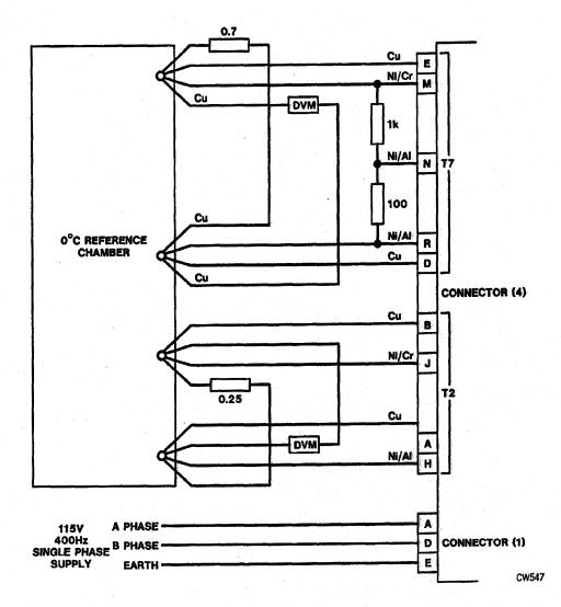
Ballasted Turbine Gas Temperature Check Figure 2
