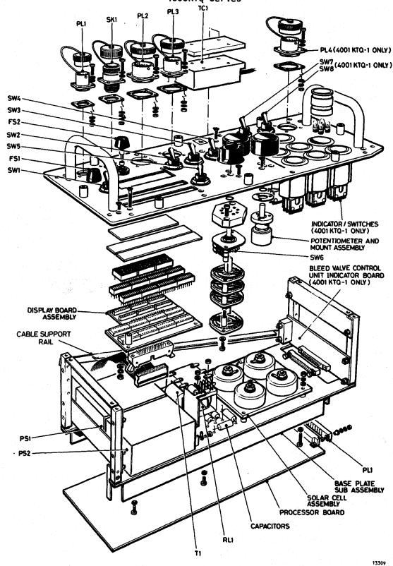
Disassembly of Testers Figure 1
