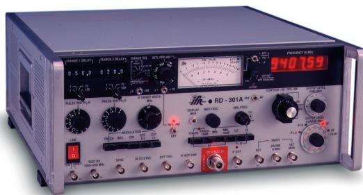
The RD-301A Weather Radar Test Set satisfies simulation requirements for new generation non-coherent radar systems
